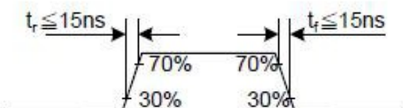
Display Serial Interface Timing Characteristics (3-line SPI system)
